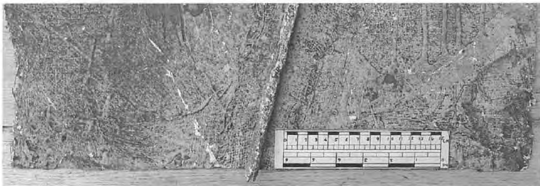
Plate 10 Front and back of typical fibrous plaster section from the Palace Theatre London, (opened 1891) showing the use of lath to provide additional reinforcement to a flat panel
