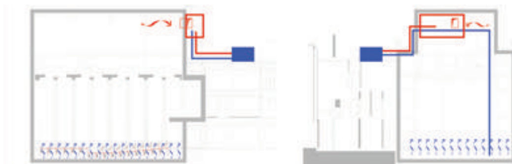
Long section and cross section showing the principle of the low-noise ventilation system
