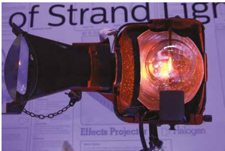
One of the cutaway lanterns, a Patt 23N, used by Strand at their King Street demonstration theatre.
