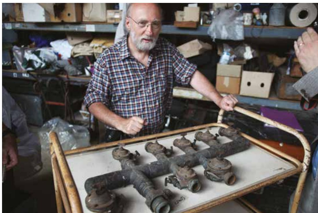
Jim Laws with a 'gas table' – a lighting desk for gas! Note the bypass valve to set a minimum 'off' level to ensure the flame stays lit even when faded out.
